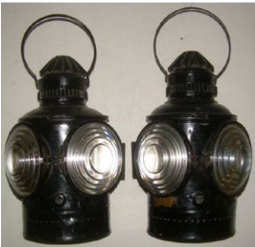
A high bid of $1050 took home this nice pair of Peter Gray & Sons classification lamps, marked for the Boston & Maine Railroad on applied tags, complete with mounting brackets, green glass panel inserts, and original fonts and burners.
