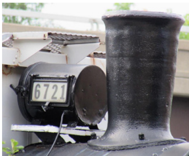
The roof walkway on the runaway covered hopper hangs over the headlight on the No. 6721, after it stopped the car in its tracks. Photo by John Koslosky from the Railroading Rambler Facebook & YouTube websites.
