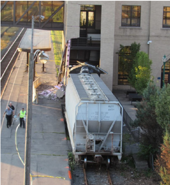
A view showing the potential for disaster if the 6721 had not been in place to stop the runaway car from penetrating the station walkway. Photo by John Koslosky from the Railroading Rambler Facebook & YouTube websites.
