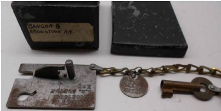
A $120 bid purchased this Slaymaker tool for checking the cut on Bangor & Aroostook Railroad switch keys.
