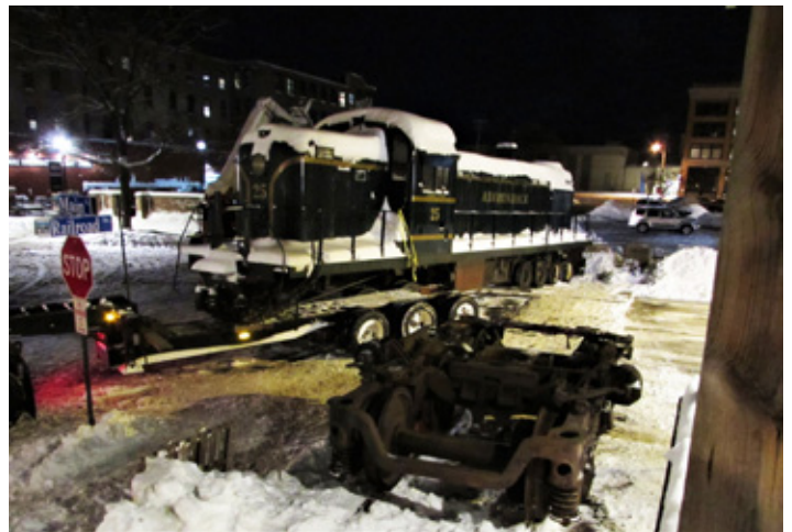
Moved from its trucks to rubber tires, Adirondack #25 awaits movement to active rails. John Koslosky photo.
