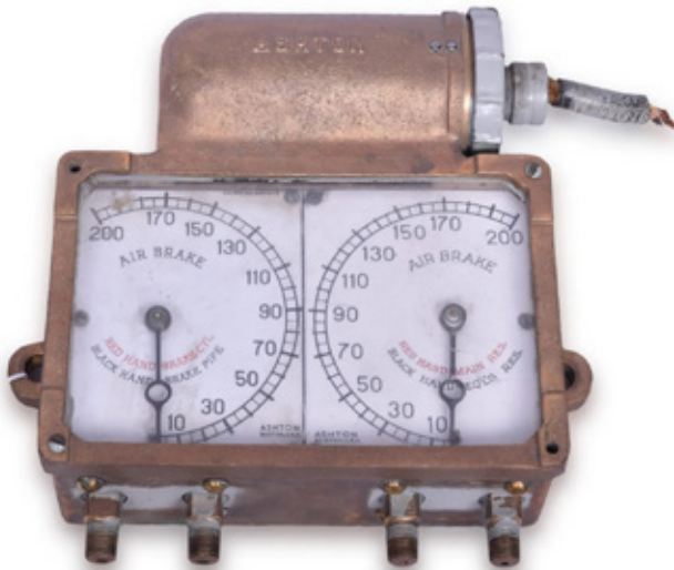
A $2500 bid bought this Ashton cast bronze dual airbrake gauge, showing main & equalizing res. and brake pipe.
