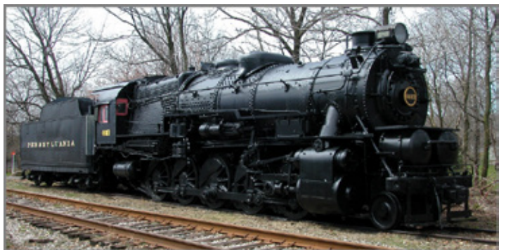
The society's cosmetically restored Pennsylvania Railroad I-1s Class Baldwin decapod steam locomotive No. 4483.
