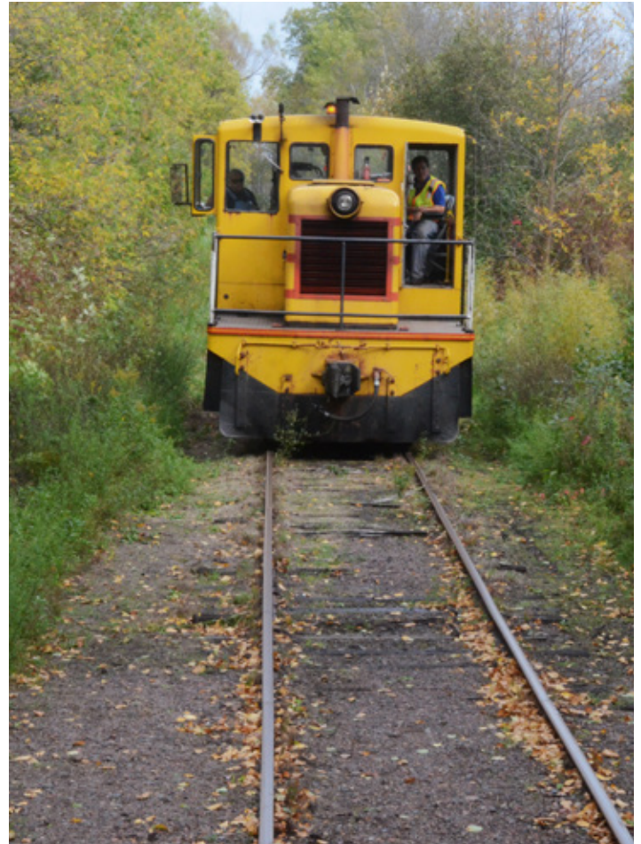
The former Flambeau Paper Co. 1946 General Electric 44-tonner prepares to tie on to the train. Author's photo.
